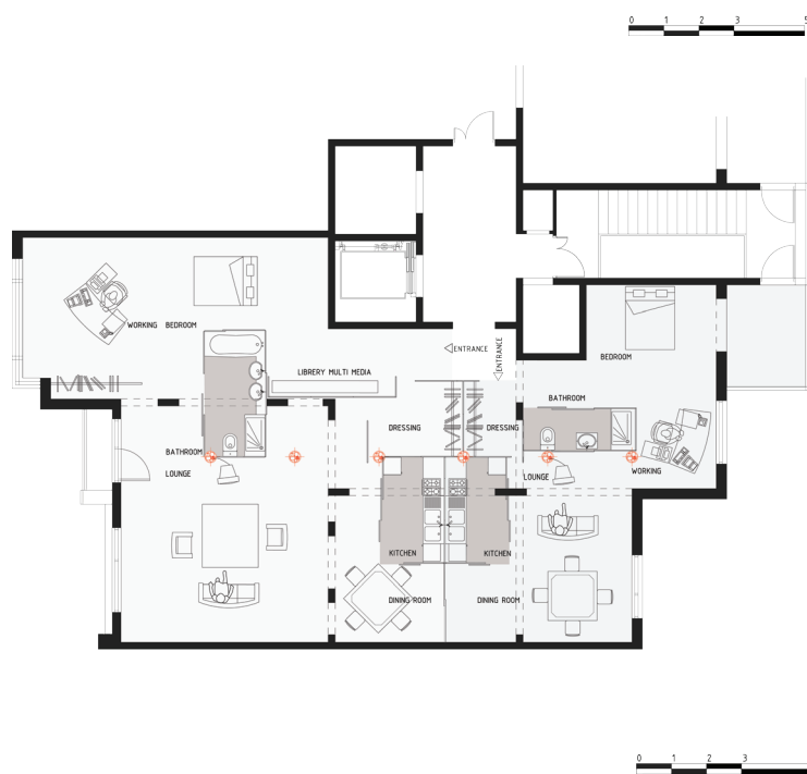
Housing developments based on drainage and supply networks that can be easily modified at the request of users
